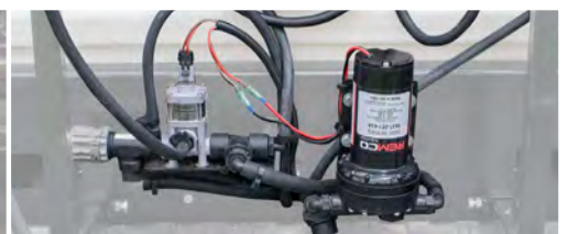
Control console Electric pump and boom control
