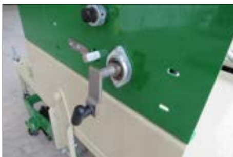
Simple & Highly Accurate Fluted Seedcup Adjustment System
