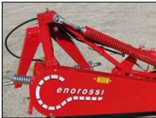
Individual Shear-hub System on cutter bar
