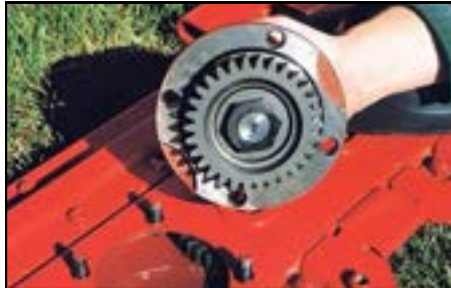
Easy changing hubs with 4-bolt disc cutting unit
