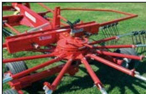
Heavy Duty, Sealed Oil Bath G-box
