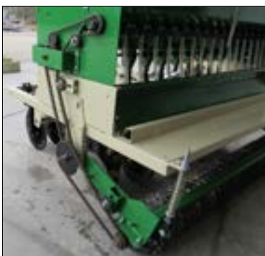
High Precision Ground Drive Seeding System.
