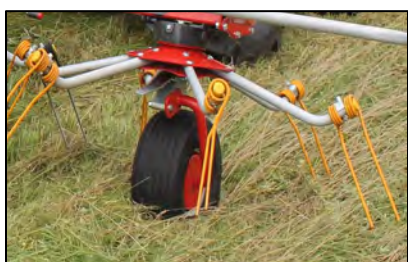
Thick-Walled Tubular Tine Arms
